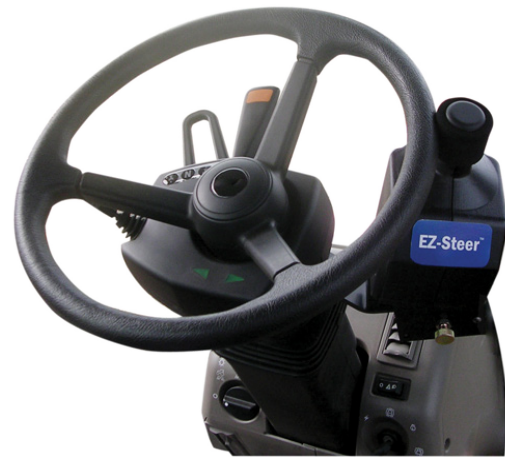
Figure 8. A Trimble EZ-Steer clamp-on auto-steer system, in which the system controls the steering wheel to keep it centered on the guidance path. Photo: Trimble Inc.
