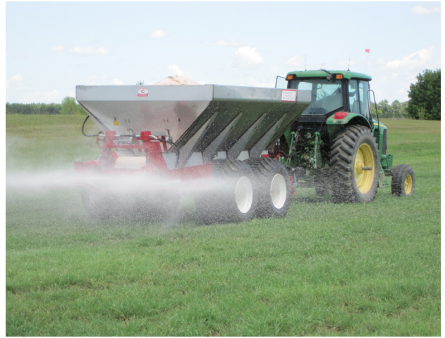
Figure 1. Example of a spinner-disc spreader application pass. This demonstrates the difficulty of determining pass-to-pass distance without skips or overlaps.
