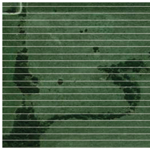
Figure 4. An example of straight guidance lines or passes across a field set at the equipment width.
